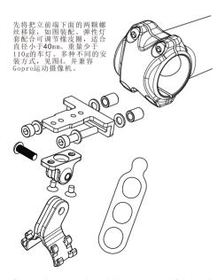
Remove the upper or lower bolts on the stem before install. Assembly as the figure. Flexible light bracket for the light diameter less than 40mm and weight less than 110g. Different kinds of installation methods. As figure 4. Compatible with Gopro.
